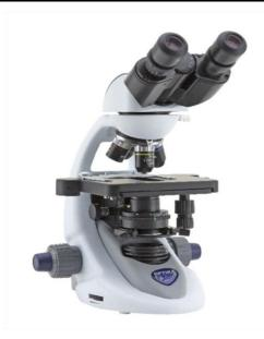
Binocular brightfield microscope, 1000x, N-PLAN objectives
